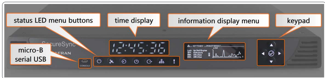
Figure 1-1: SecureSync front panel layout
