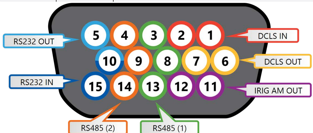
Figure 2-20: Multi I/O 15-pin connector, in mating direction from front
