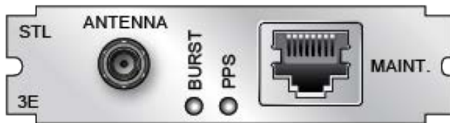
Figure 5-63: Model 1204-3E option card rear plate
