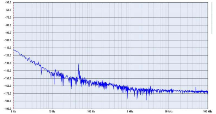
Typical MO ULN Phase Noise at 10MHz
