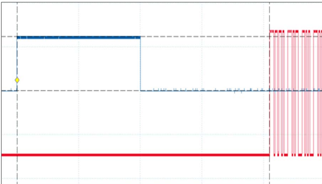
Figure 8-5: Configuration 2: Timing offset=20ms. 1PPS in blue and NMEA messages in red.
