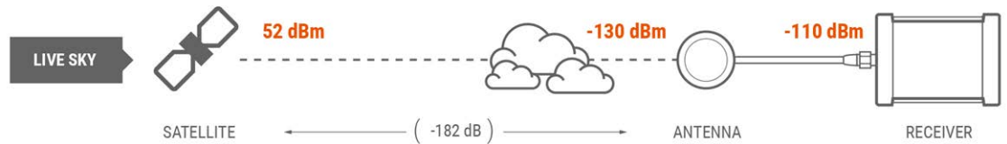
Figure 1-1: Propagation of the real GNSS signal from the satellite to the GNSS receiver
