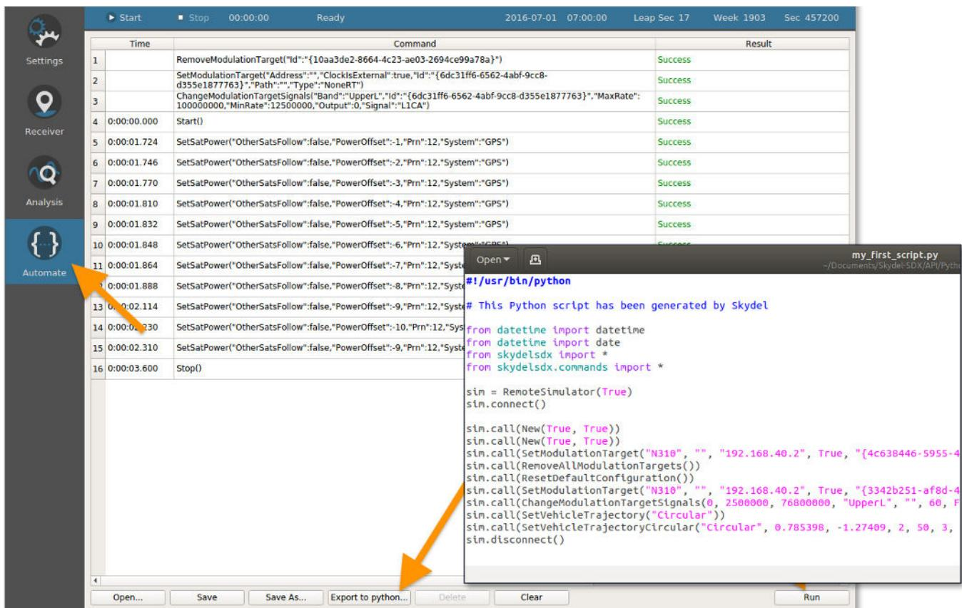
1. All Skydel actions are transformed into Commands and logged into the Automate tab.
