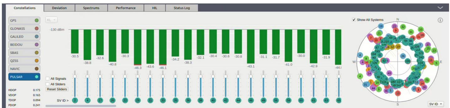
This **Constellations** subtab displays information about the GNSS satellites that are simulated and is divided by constellation and SV. Satellite power control as well as a Skyview allows you to define the strength if the satellite's signal and see its position.
