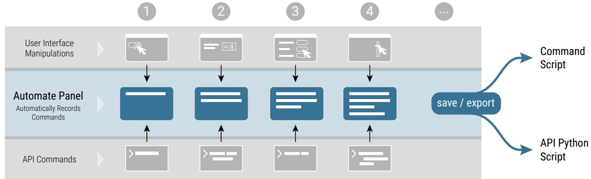
**Automate:** Skydel was built around the Command Design Pattern, which means that all actions (either from GUI or remote control) are sent to the engine using commands. The commands are processed by the engine exactly the same way whether they come from the GUI or remote program. If your simulation is working via GUI, it will work exactly the same via the API.
