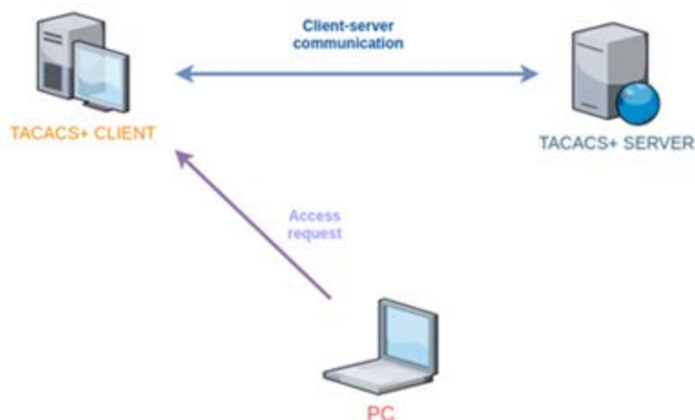
Figure 6-2: TACACS setup for verifying the installation.
