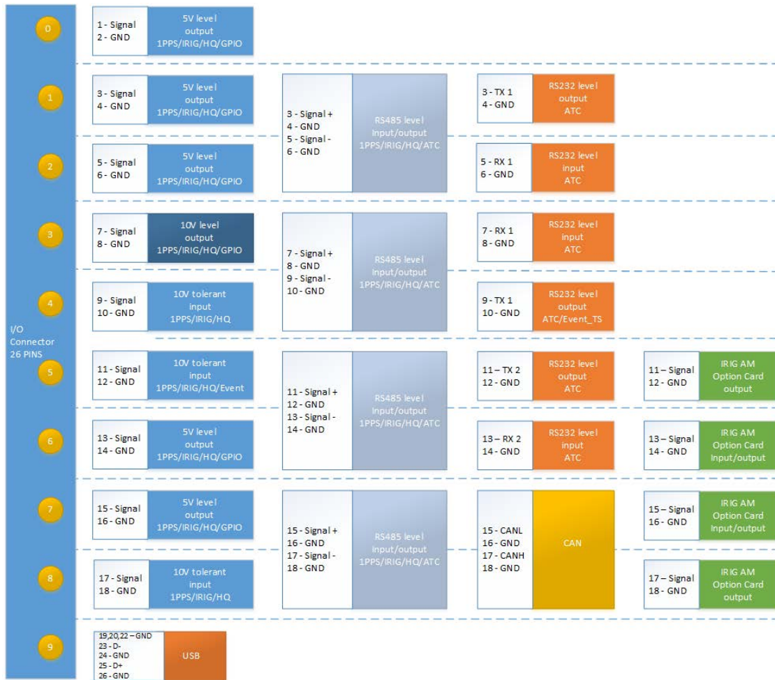
Figure 5-3: VersaSinc Pinout (IRIG AM Option Card in Green)
