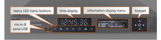
Figure 4-1: SecureSync front panel
