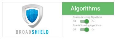
This menu option allows you to disaable/enable Jamming or Spoofing. **Spoofing** refers to impersonating the live-sky GNSS signal, thus "deceiving" the GNSS receiver, while **Jamming** refers to interference of the signal, i.e. making the live-sky GNSS signal unusable. Per default, both are Enabled.
