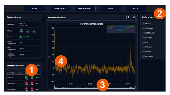
On the left side of the screen, **Status** information is displayed for the System and the References. Note that the **Reference Status** panel also displays the latest PHASE OFFSET reading (1) for active references against the System Ontime Point. The reading is updated every 30 seconds.
