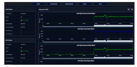
Navigate to TOOLS > SYSTEM: Ethernet Monitor. The Ethernet monitoring screen opens:
