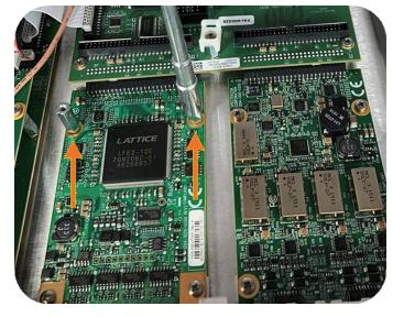
Figure 5-8: Bottom card with standoffs installed
