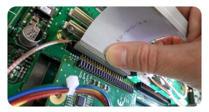
Figure 5-9: Ribbon cable installation
