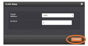
Your new VLAN interfaces will now be displayed in the VLAN Setup panel, listed as eth[#].[VLAN ID].
