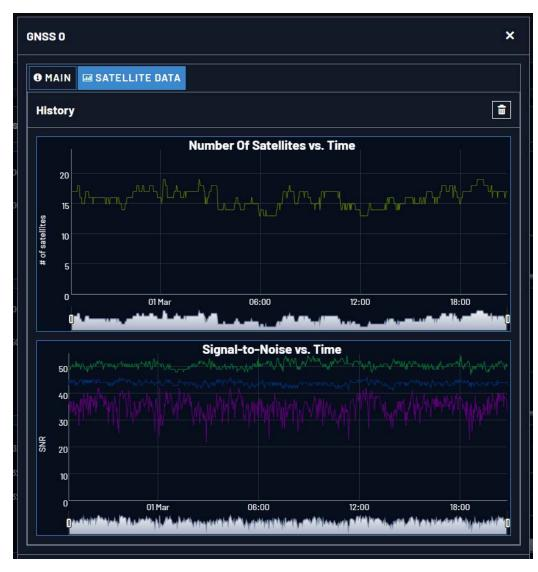
In both graphs, to see a legend of the graphical data, and time-specific status data, click inside the graph, choosing the desired point in time. If necessary, increase the time resolution by dragging the time sliders. A pop-up window will display the legend for that graph, and the status information for the selected time.
