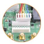
Figure 5-11: J19 Connector, seen from rear of unit.
