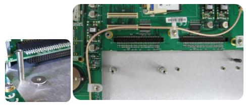
Figure 5-6: Washers & standoffs secured to chassis screw holes
