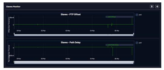
The Datasets and Statistics buttons will also provide information about the frequency of packet exchange, and the state of timing in the nodes that the PTP port is communicating with.
