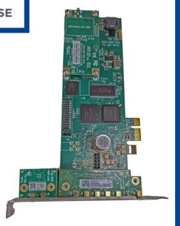
Safran's CDM-7 clock distribution and timing reference module is a PCIe card that provides 10MHz and 1PPS signals for up to seven devices that need precise synchronization.
