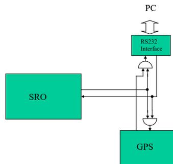
Figure 2 - Communication Diagram (Switch S6 to the left)
