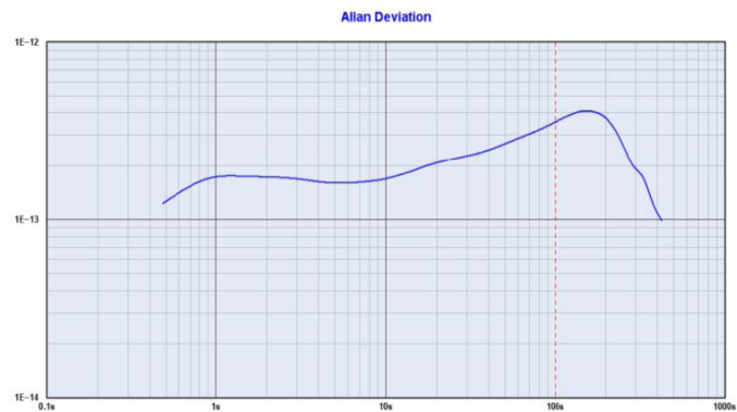
Typical MO LN Allan Deviation at 10MHz
