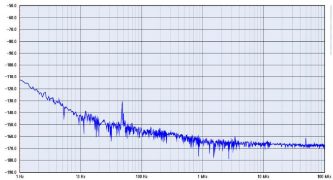
Typical MO LN Phase Noise at 10MHz
