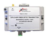
When fiber optics are required for connection between a Safran GPS receiver device and a roof-top antenna, we offer the Optical Zonu GPS over Fiber Optic Link Kit. The link between the fiber transmitter and receiver is via 9/125 micron singlemode simplex fiber via SC/APC connectors up to 5 miles (8 km).
