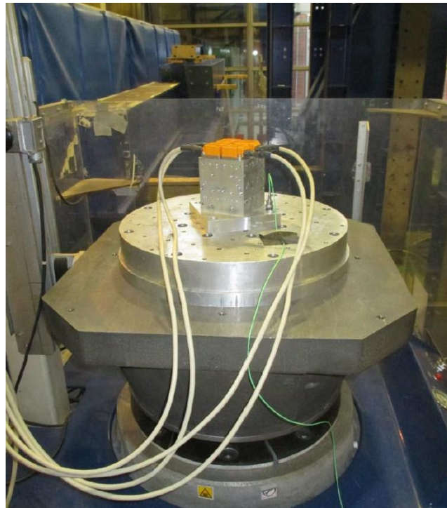
Figure 17: Test set-up for shock tests #3 and #4 (testing in z-direction)
