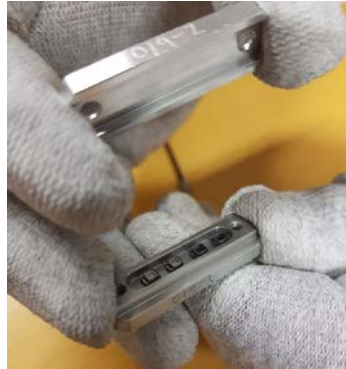
Figure 2. Special test-fixture for high-g static load
