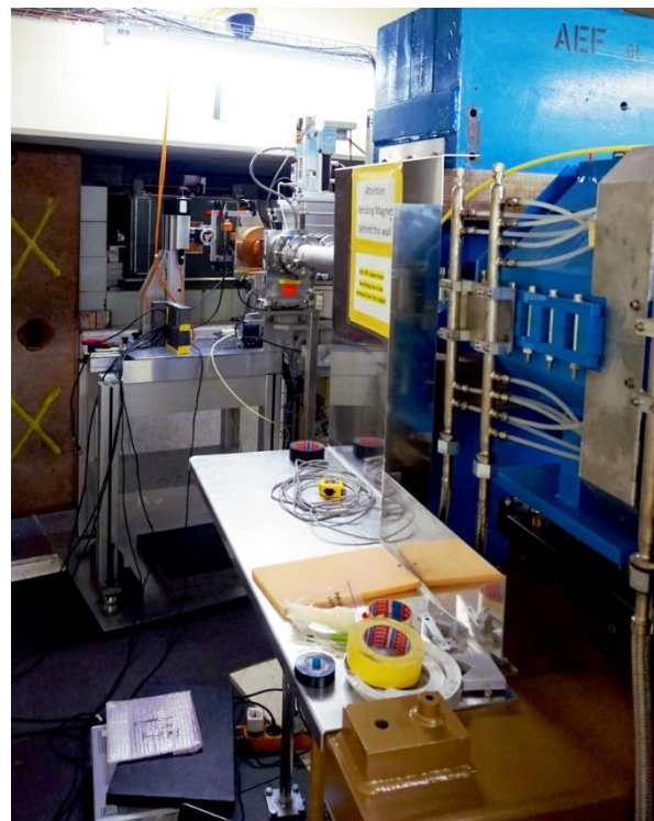
Figure 9: Single-Event Effect test set-up
