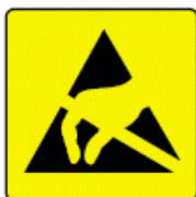
*Observe all ESD procedures when handling the board and the computer. Before installing the board, discharge static buildup by touching the metal frame of the computer with one hand and the protective bag containing the board with the other hand. Open the protective bag only after static buildup has been safely discharged.*
