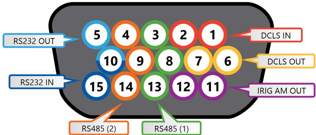
Figure 1-5: Multi I/O connector, viewed in mating direction on rear of unit
