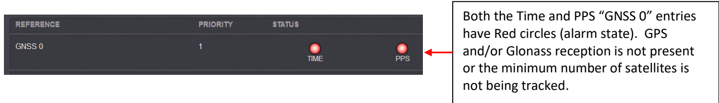
Figure 3: Input Reference Status page with GPS reception either not present or invalid
