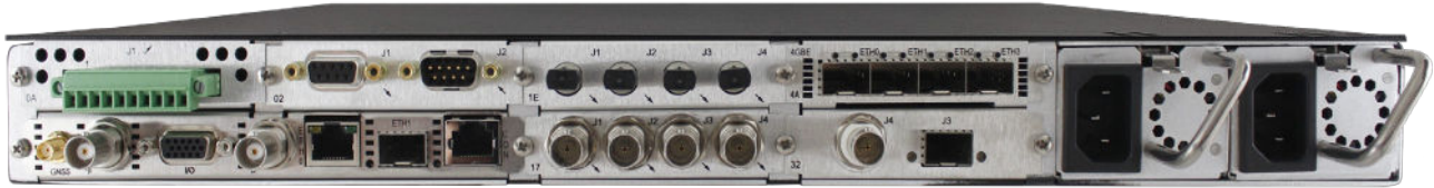
SecureSync 2400 Add the features you need through options modules, up to 6 option modules per unit and 2 Hot Swap power supplies slots.
