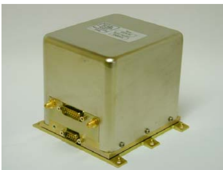
Figure 1. Picture of the updated RAFS1 once closed including the thermally regulated base plate
