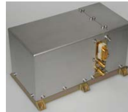
Figure 1. Picture of space RAFS (3.2kg) for Galileo GNSS
