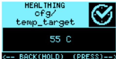
To exit this screen, long press over INFO/CTRL button. To go to next parameter, short press over INFO/CTRL button. When the last parameter was reached, a short press over INFO/CTRL exits this screen, returning to the previous menu.
