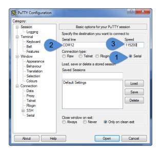
Figure 3-2: Putty configuration for serial port connection.
