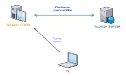
Figure 6-2: TACACS setup for verifying the installation.
