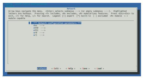
3. Then the corresponding network interface (eth0) to be modified must be selected:.
