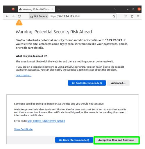
Figure 9-1: Accepting an untrusted certificate in Firefox.
