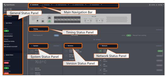
Figure 4-3: Web GUI Dashboard sections
