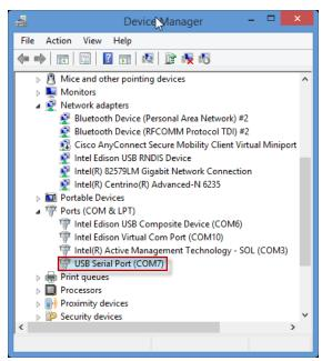
Figure 3-1: Device manager. New serial port detected.
