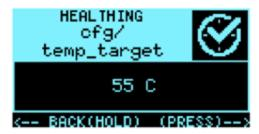
To exit this screen, long press over INFO/CTRL button. To go to next parameter, short press over INFO/CTRL button. When the last parameter was reached, a short press over INFO/CTRL exits this screen, returning to the previous menu.
