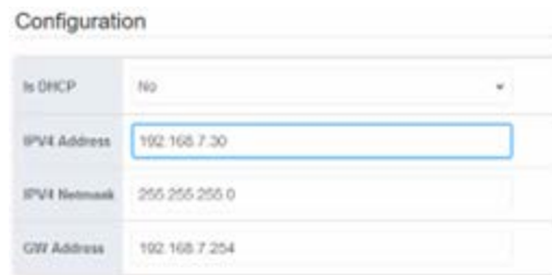
Figure 4-5: Configuration of static IP using web interface
