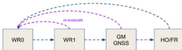
Figure 5-1: Multi-timing sources handle by FOCA policy with its two strategies: only fall-down (blue) & re-evaluation (purple)
