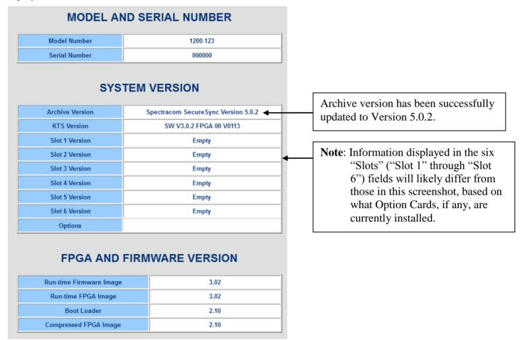
Figure 10: Example "System Version" information upon completion of the update
