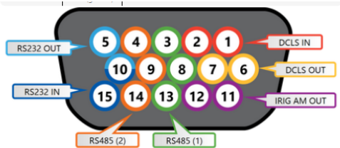
Multi I/O 15-pin connector, in mating direction from front
