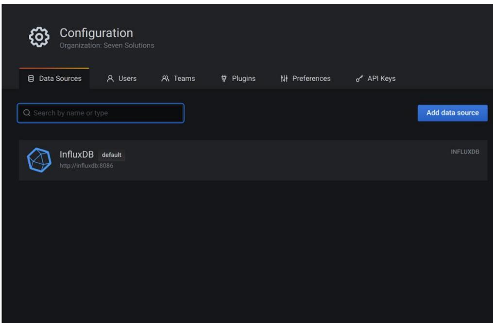
Press in the InfluxDB data source and set the token in its configuration. Then, press the **save & test** button. The correct configuration shows the following message:
